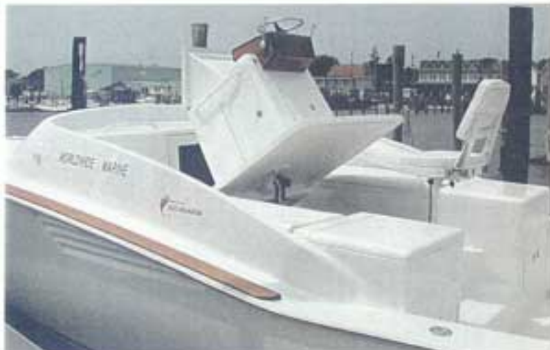
The helm pod lifts with the flick of a switch to provide ready access to the wide-open engine compartment below.
